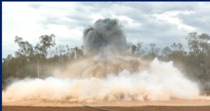
Figure 1: Video images from a series of instrumented, unconfined 40 -50 kg blasts of a stabilised H_2O_2 / mineral oil-based emulsion explosive (Rurex).
