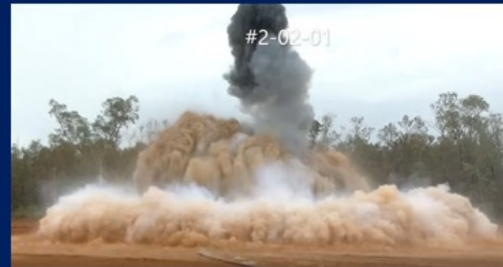
Figure 1: Video images from a series of instrumented, unconfined 40 -50 kg blasts of a stabilised H_2O_2 / mineral oil-based emulsion explosive (Rurex).
