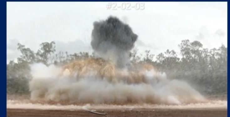
Figure 1: Video images from a series of instrumented, unconfined 40 -50 kg blasts of a stabilised H_2O_2 / mineral oil-based emulsion explosive (Rurex).
